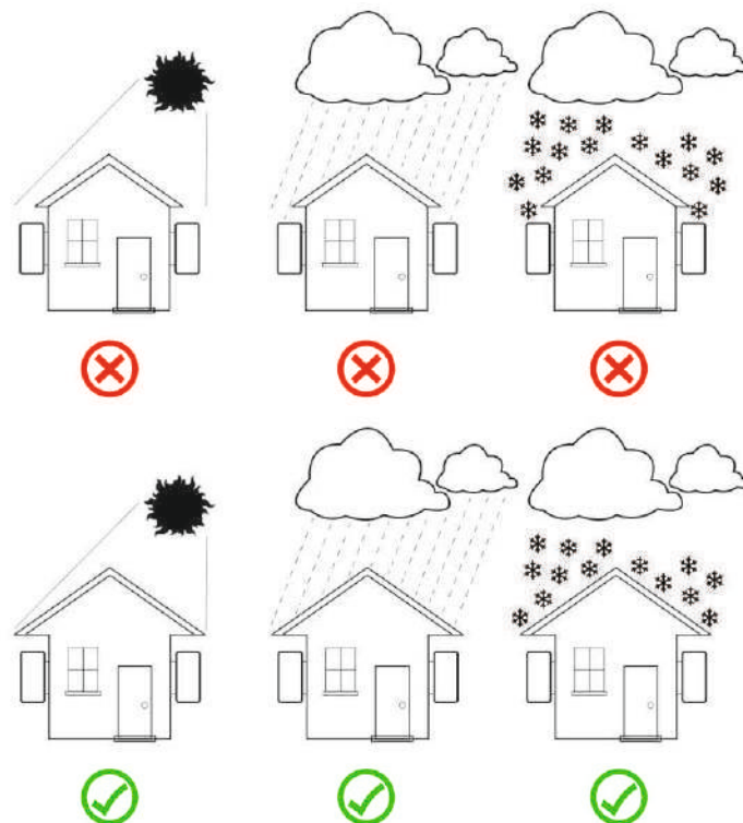
Pic 4.1 Recommended installation place
