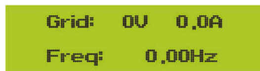
Pic 8.4 AC running state information
