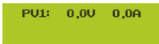
Pic 8.3 PV input voltage and current information
