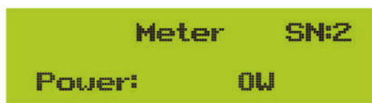
Pic 7.3 Parameter setting When the EASTRON meter connected successfully, it will shows SN: 2
