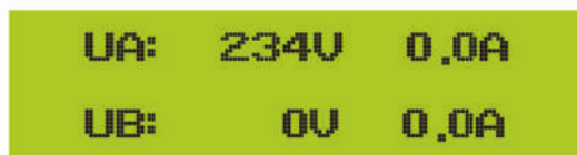
Pic 8.5 Grid voltage and current information
